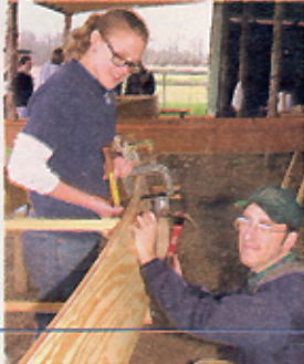
Novice boatwrights learn to bend and nail wooden boards.
