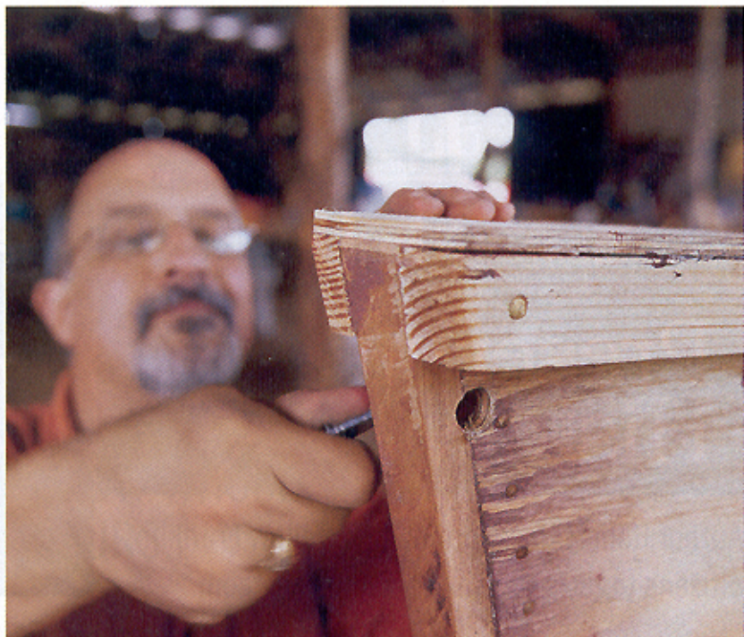
above: Glue and nails hold together each piece of wood, sealed with waterproof caulk. below: Karl and the writer maneuver for position in their newly built boats. These Bevins skiffs are products of the two-day boat school.
